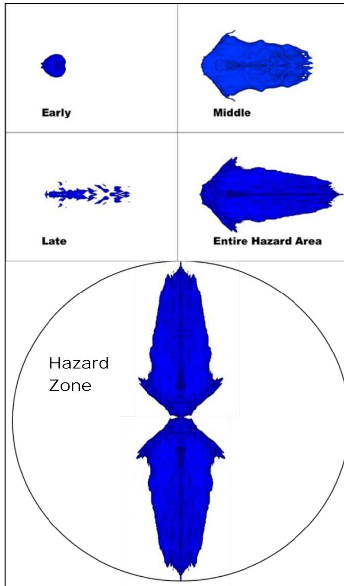
**Figure 2: Time-Dependent Vapor Dispersion<sup>14</sup>**
